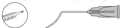
7527 LASIK Irrigator - Assis - 3 Ports 27G x 7/8 in (.40 x 22mm) Formed 9mm from end Tip flattened 1.5mm from end One .15mm port 2mm, 4mm and 6mm from end
