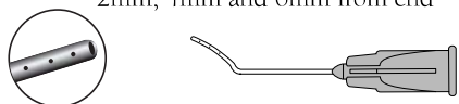
7727 LASIK Irrigator - 6 Ports 27G x 7/8 in (.40 x 22mm) Formed 9mm from end. Two .15mm ports 2mm, 4mm and 6mm from end
